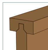
If measured and cut correctly, the Easy-Fit Top Cap should finish flush on the shoulder of the top board as pictured.
